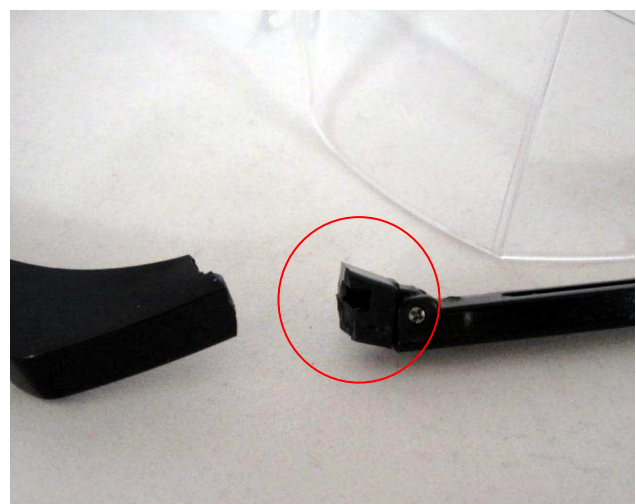
Figure 2: Sample 17206-20, fixture of frame to lenses breaks caused by impact at 45 m/s.
